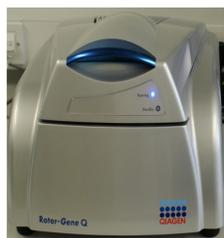
Figure 1: Rotor-Gene Q thermocycler
